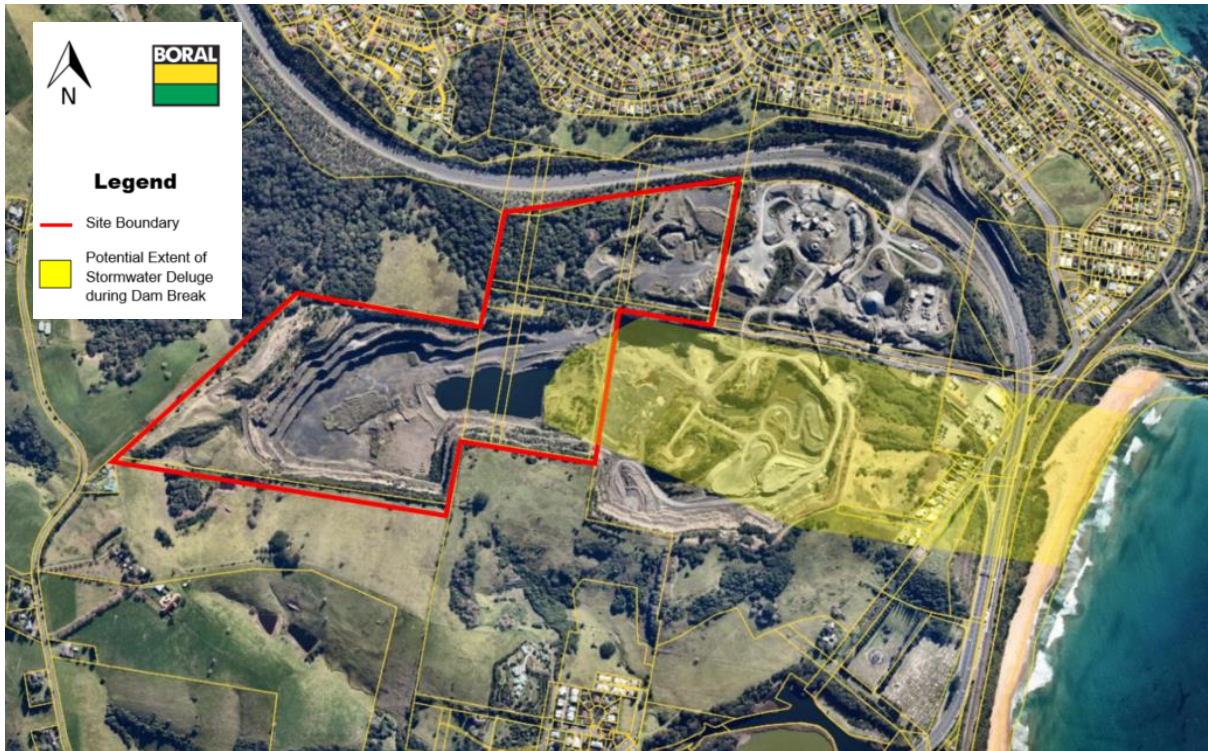
Figure 8: Incident 3: Overflow of Sediment Dams due to Flooding or Dam Failure
