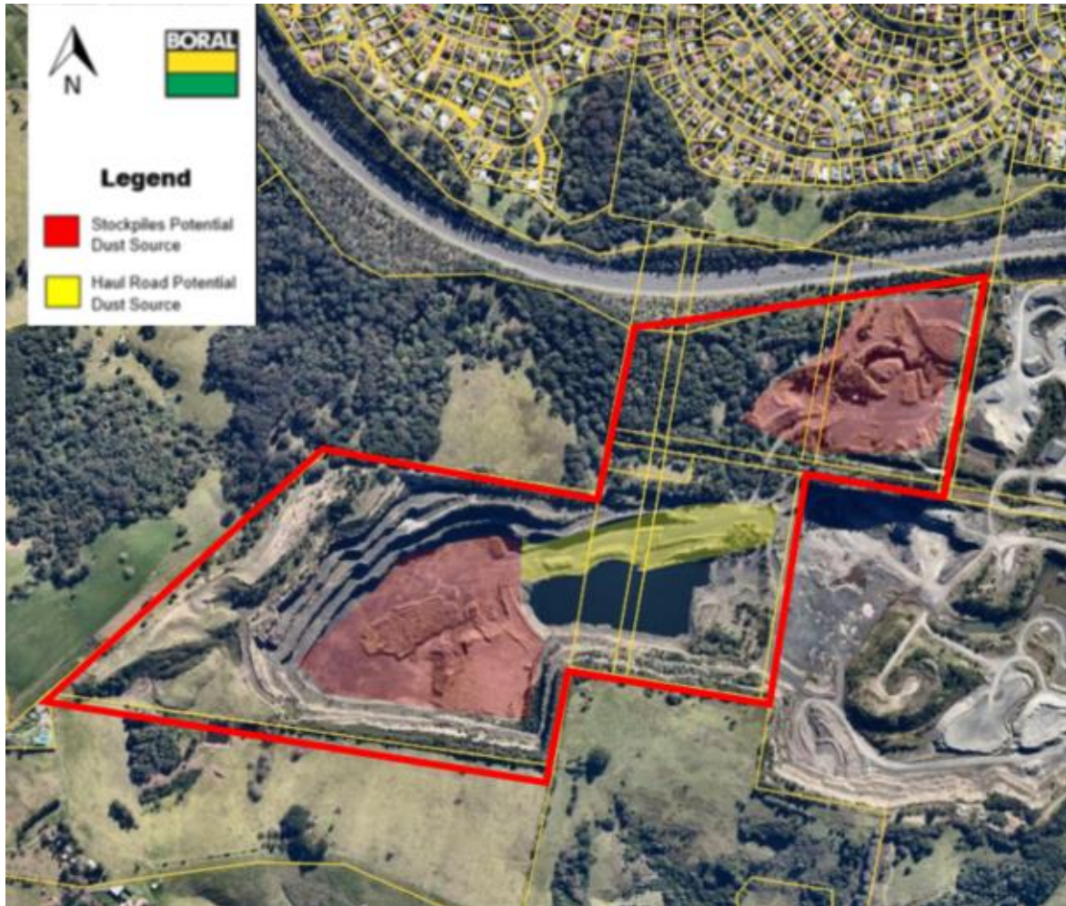
Figure 6: Incident 2: Sources of Dust Pollution at Bombo
